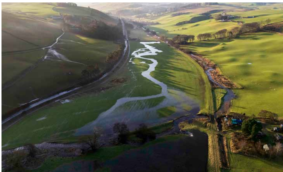
The Eddleston Water in high flows – we can clearly see where the river wants to be but for the last 200 years it has been pinned behind the railway line to the right
