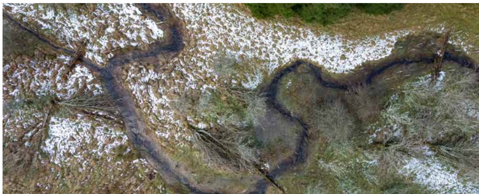
An aerial view of the Middle Burn in the Eddleston Water catchment, host to a number of log jams/lateral flow deflectors which play an integral part in delaying flood peaks and giving people more time to prepare for the impact of flooding
