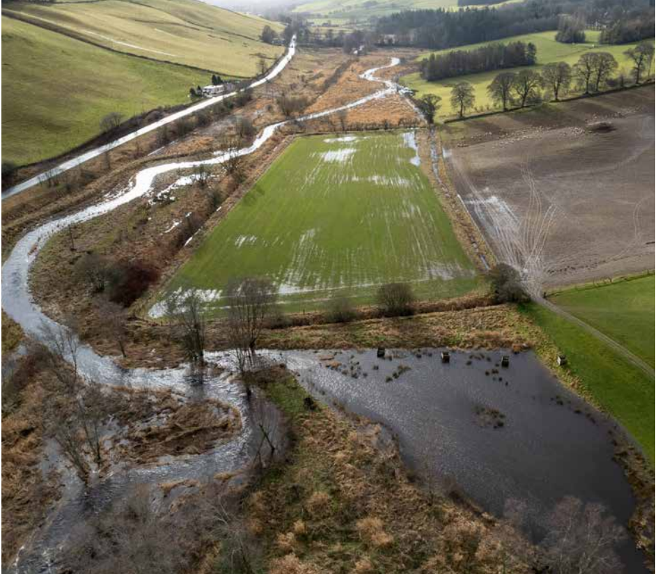
NFM measures to "slow the flow" of water include re-meandering and flood storage ponds (bottom right of image)
